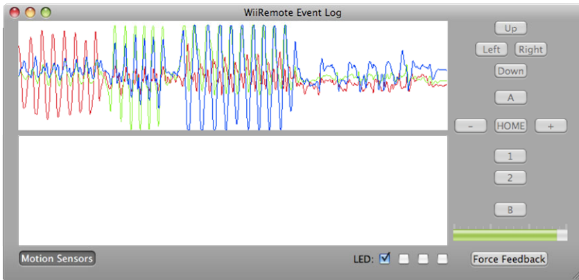
Fig. 1. Screenshot from DarwiinRemote-Software Showing Readings from Accelerometers
