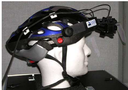
Figure 2: The mobile eye-tracker
